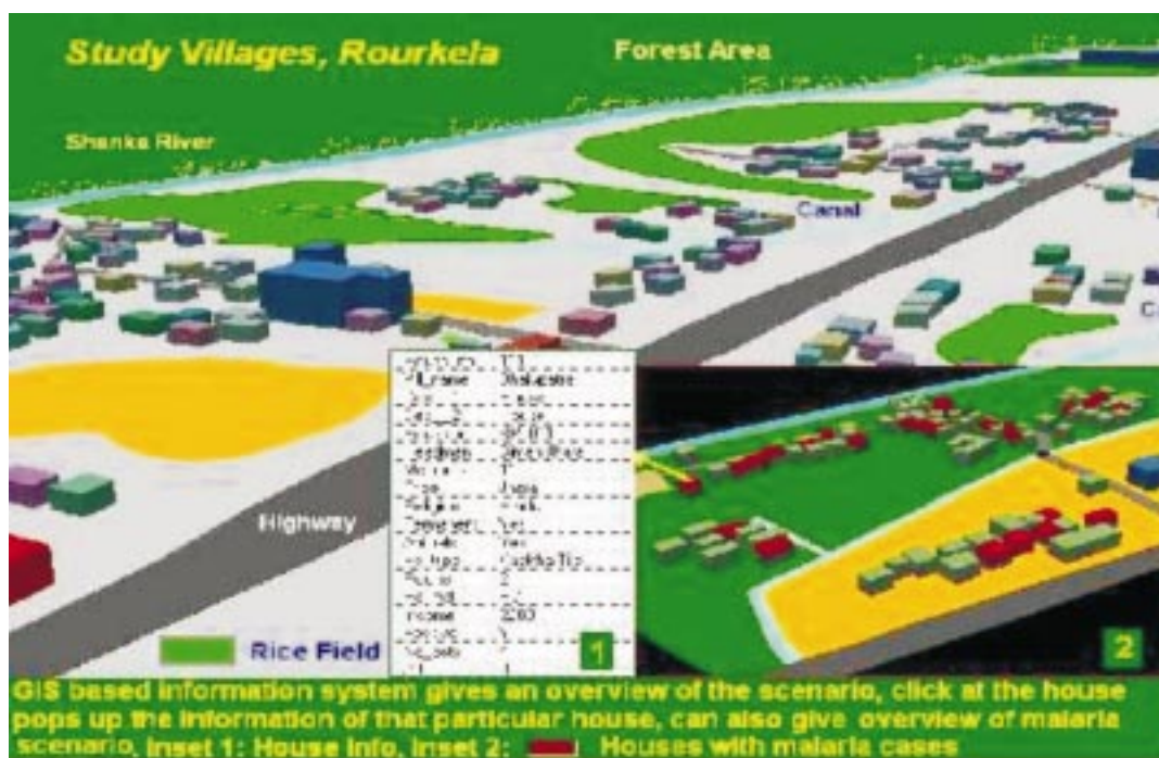
Fig. 19: GIS-based information system consisting of three tier information on village, house and personal level
